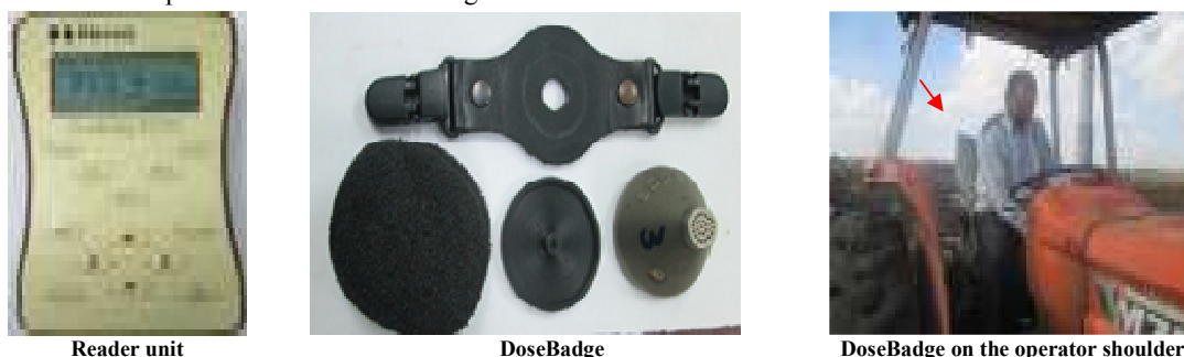
Fig. 2. Reader units RC 110A and doseBadge CR:110A positioned on the operator shoulder.
